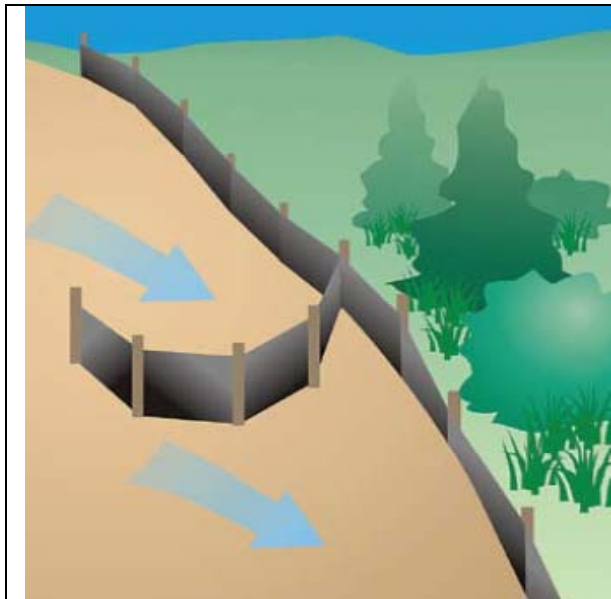
"J-hooks" used during silt fence installation ▲
