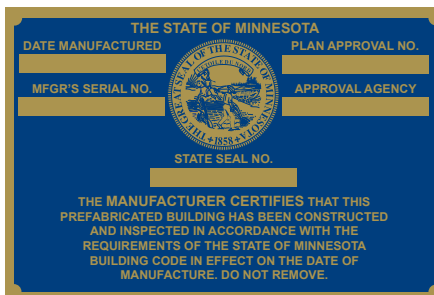
Example prefab construction label - located under kitchen sink.
